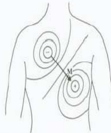
Figure 6.1 Rough sketch of the dipole field of the heart when the R wave is maximal. The dipole consists of the points of equal positive and negative charge separated from one another and denoted by the dipole moment vector M .
