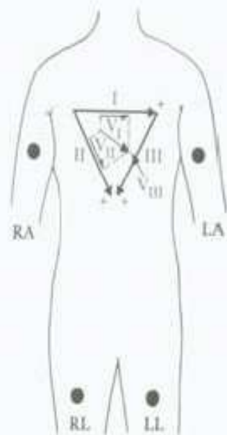
Figure 6.3 Cardiologists use a standard notation such that the direction of the lead vector for lead I is 0^\circ , that of lead II is 60^\circ , and that of lead III is 120^\circ . An example of a cardiac vector at 30^\circ with its scalar components seen for each lead is shown.
