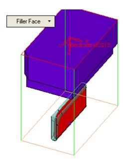
A filler face has been applied to the side of the electrode.
