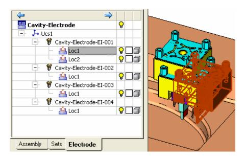
By pressing and holding the Ctrl key more than one electrode can be picked, the result being a new sheet created in the drafting environment, for each electrode.
