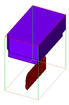
The chamfer has been created using the default preferences option i.e. the corner closest to the reference UCS.
