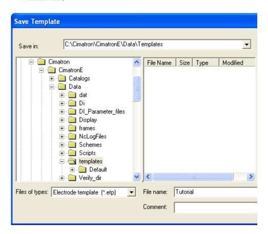
A template can hold one or more of the following features, which have been created in the electrode document: Blank, Electrode UCS, Holder, and Extension features.
