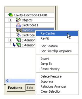
The Re-Center and Re-Fit operations update the Blank feature, considering any new geometry created.
