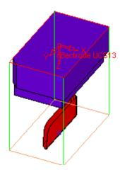
The Electrode UCS was automatically orientated for machining.
