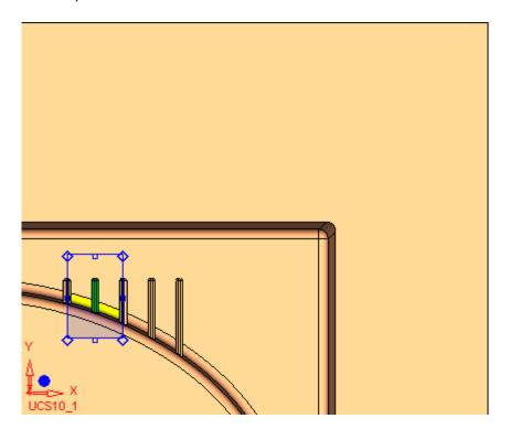
Attach the faces to the electrode and change the No Template option to **Apply Template**.
